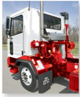
Features most spacious cab interior for driver and passenger comfort 6'4" Great chassis for automated side loader refuse applications 19" first step 32.75" second step
